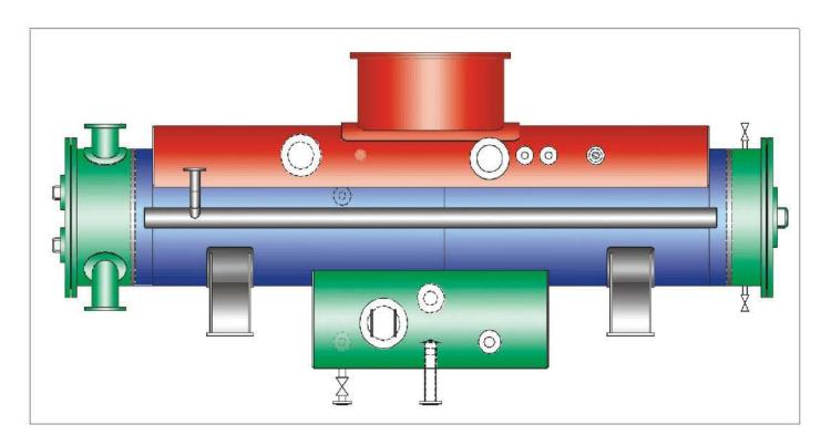
Our condensers feature high overall heat transfer coefficients (which result in smaller heat transfer areas and thus optimal use of the available space) and extremely low oxygen concentrations in the condensate. They are designed to stand up to turbine and steam generator overloads and to variations in cooling water temperature at different times of the year.
