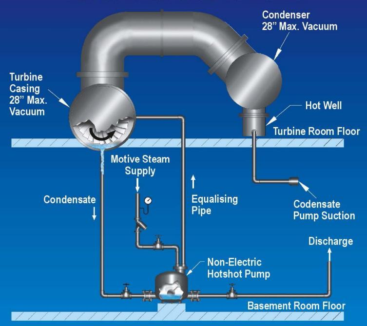
Condensate removal from turbine casing to increase turbine life and power plant performance.
