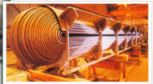
L.P. Heater under fabrication for 10mw power plant.
