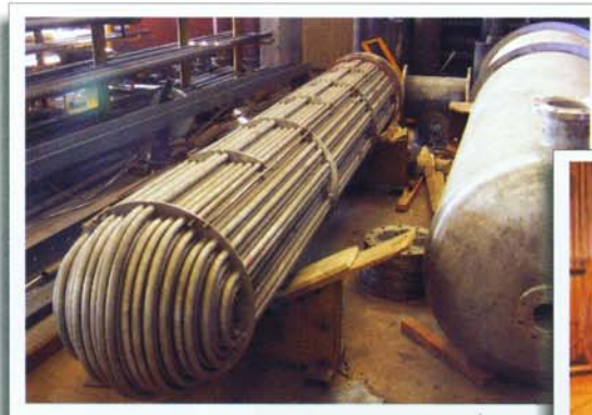
H.P. Heater under fabrication for 40mw power plant.
