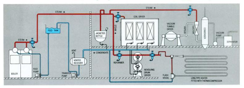
On any steam distribution system Reformer can help you achive maximum efficiency and save energy all along the line
