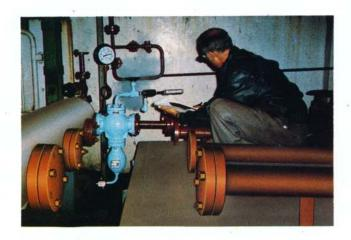
Separation efficiency test conducted in our in-house steam test facility with Croll-Reynolds Company, Inc. USA Steam Calorimeter.
