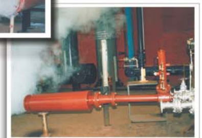
Silencer under test for a start-up ejector to ensure operation at minimum noise level in accordance with OSHA mandated noise exposure limits.
