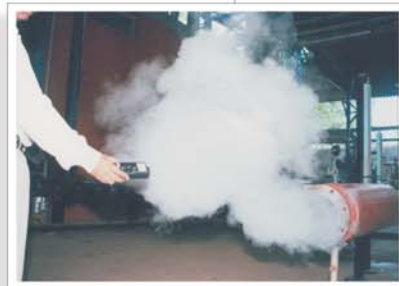
Silencer under test for a start-up ejector to ensure operation at minimum noise level in accordance with OSHA mandated noise exposure limits.
