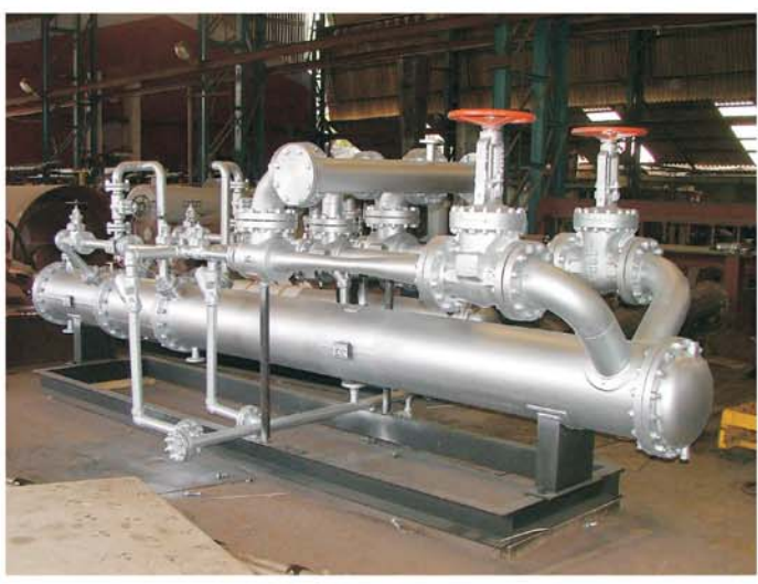
Croll-Reynolds Steam Jet Evactor Systems, model No. CR Series-200S above and 300S below for Turbine Extraction manufactured in India by Mazda Limited.
