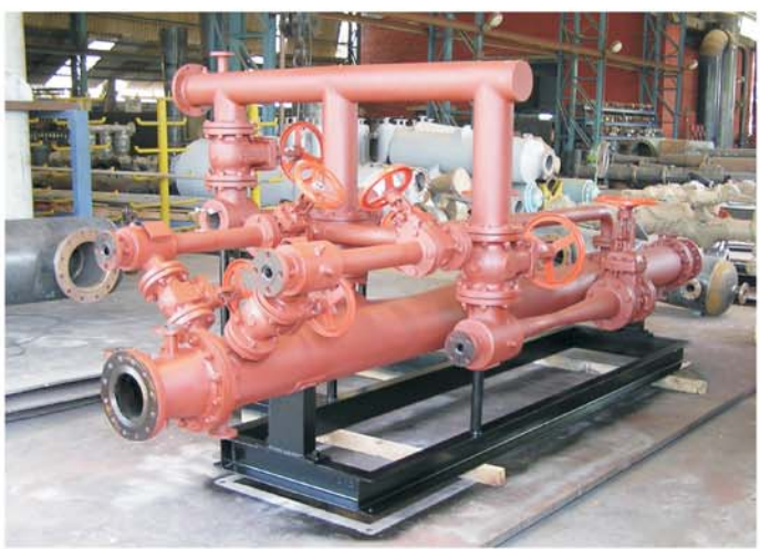
Croll-Reynolds Steam Jet Evactor Systems, model No. CR Series-200S above and 300S below for Turbine Extraction manufactured in India by Mazda Limited.
