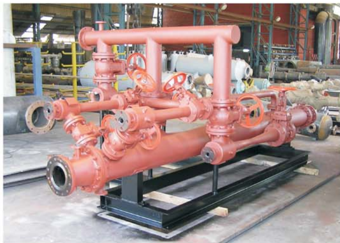
Croll-Reynolds Steam Jet Evactor Systems, model No. CR Series-200S above and 300S below for Turbine Extraction manufactured in India by Mazda Limited.
